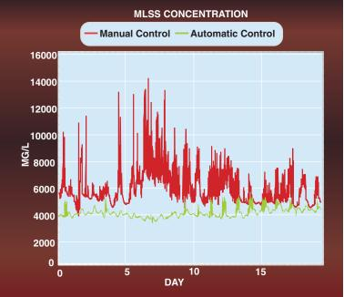
Suspended solids concentration has less variability due to SRTMASTER's ability to measure TSS and calculate wastage on-line. As a result, clarification is improved, especially during peak and storm flow conditions because solids mass loading on clarifiers is reduced.
