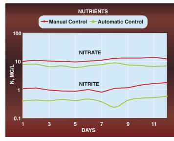
Under constant SRT, nutrient removal is improved because ammonia removing authotrophs and denitrifying heterotrophs function under optimum conditions.
